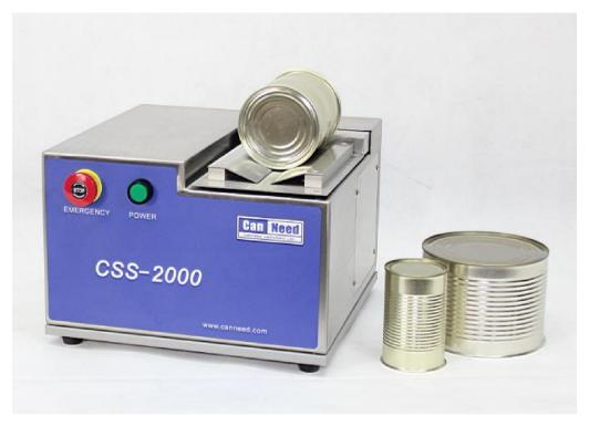
"CanNeed-CSS-2000 Seam saw" is a special seam circular saw with double cut for double seam inspections. The CanNeed-CSS-2000 was specially designed for 2- and 3-piece cans. The nitrated blades achieve together with the speed of approx. 1.000 r/min. a very plain cut surface. The seam image on CanNeed series Automatic Seam Computer (Video Seam Monitors), and automatic seam measuring systems gets thereby very clear and improves measurement speed and reliability.
